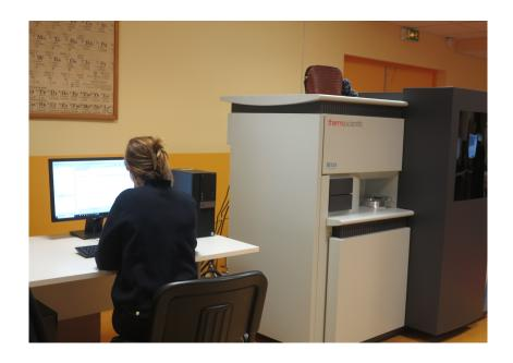
The Escalab 250 Xi device offers a very high energy resolution. A helium lamp allows measurements of UV spectroscopy (UPS) giving access to the valence bands. The use of Helium light ions makes it possible to access the composition of the first atomic layer (Low Energy Ion Scattering). A REELS module (Reflection Electron Energy Loss Spectroscopy) allows in particular to access hydrogen, non-probed element by XPS spectroscopy.
