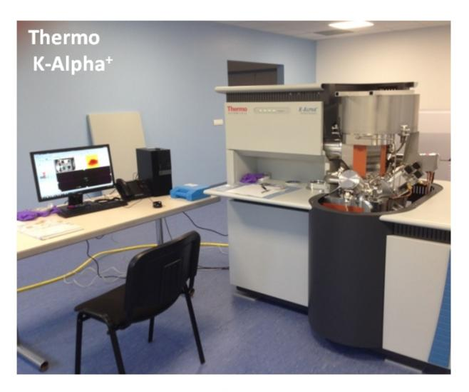
XPS: Chemical environment and composition + Profilage (Ar+, Ar<sub>n</sub>+)
