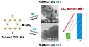
nm) in a very homogenous fashion, using the double solvant (DS) method. Unlike the impregnation method (IM), the DS method produces materials with remarkable catalytic activities, among the highest reported to date for catalysts derived from MOFs (under revision for ACS Applied Materials and Interfaces).
